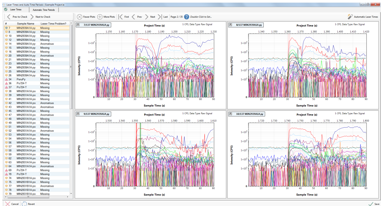
Figure 48: Laser Time window for a Project with many problematic time values. The shaded regions show the median relative time period ( \pm a standard deviation value) for all laser times in the Project. In a situation like this where many laser times have been missed it will be best to adjust the settings. What to do About Missing Ablations?
