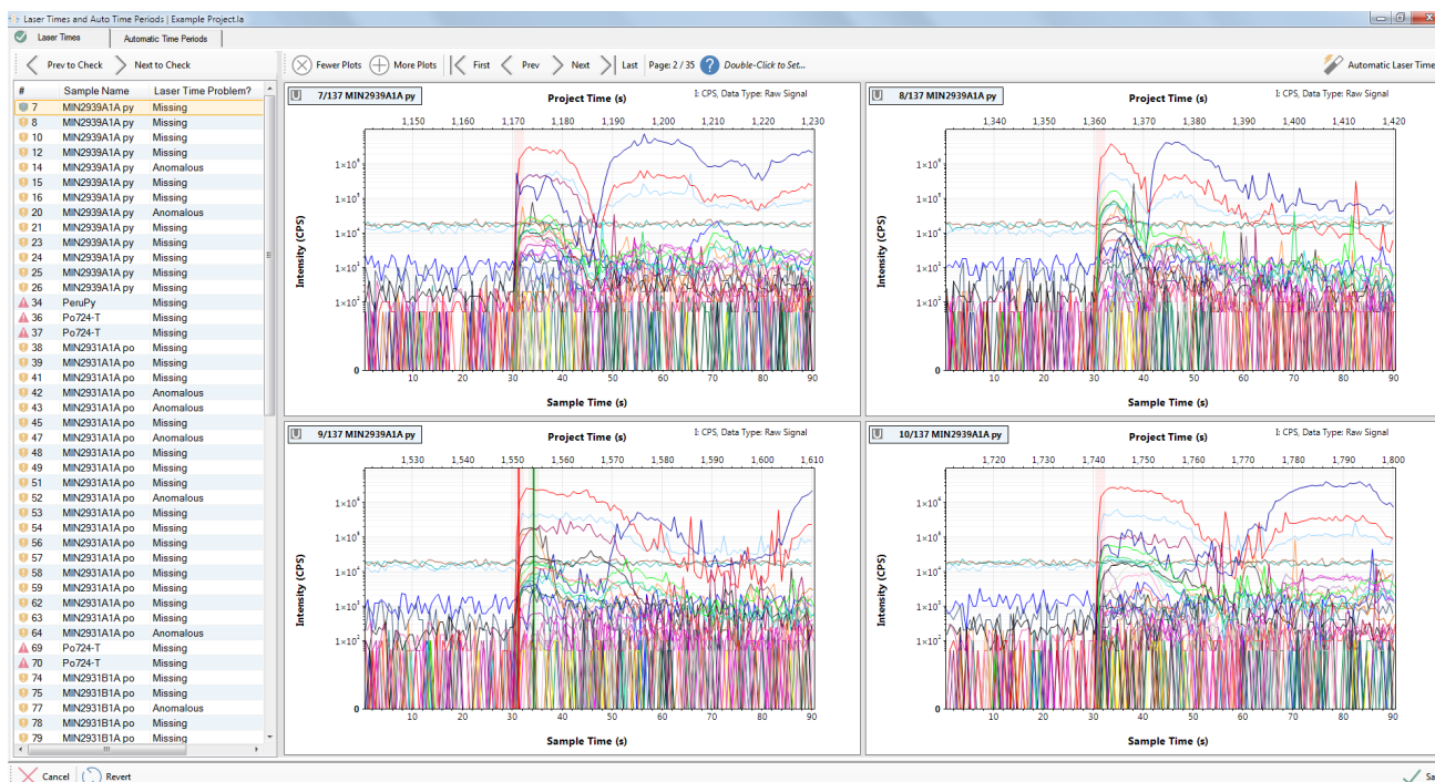
Figure 45: Laser Time window for a project with many problematic time values. The shaded regions show the median relative time period ( \pm a standard deviation value) for all laser times in the project. In a situation like this where many laser times have been missed it will be best to adjust the settings.
