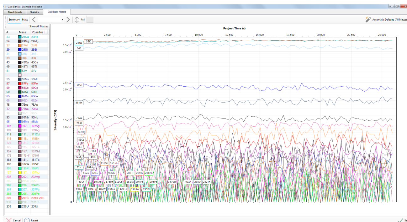
Figure 57 "Gas Blank Models" tab showing the mean value of each gas blank time period for every mass over the entire project.
